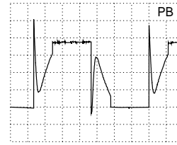
DC, 2V/Div, 1ms/Div Connector 1930-(1), -(2), -(3) ⑤⑥
